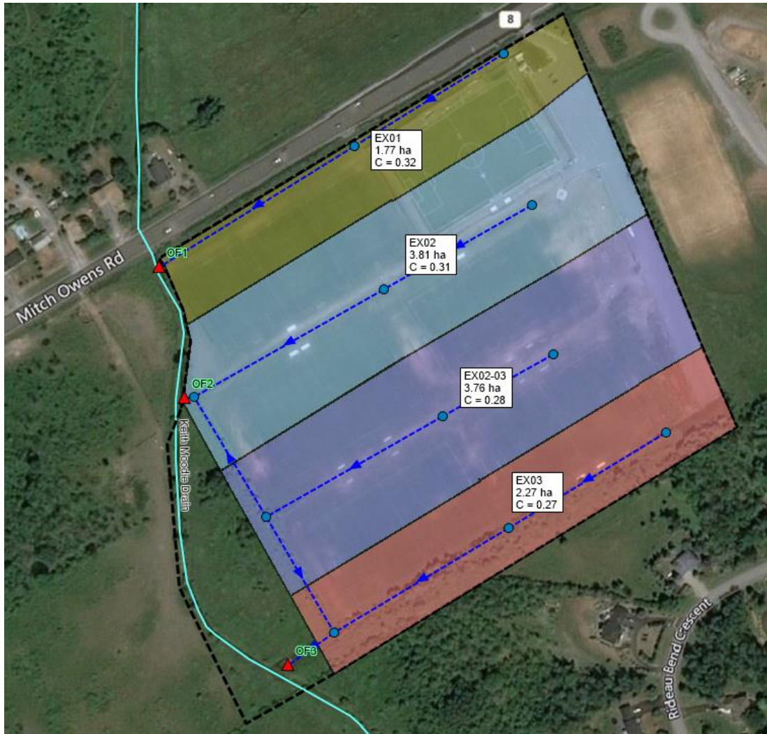
Figure 2: Existing Conditions Catchment Areas and Runoff Coefficients
