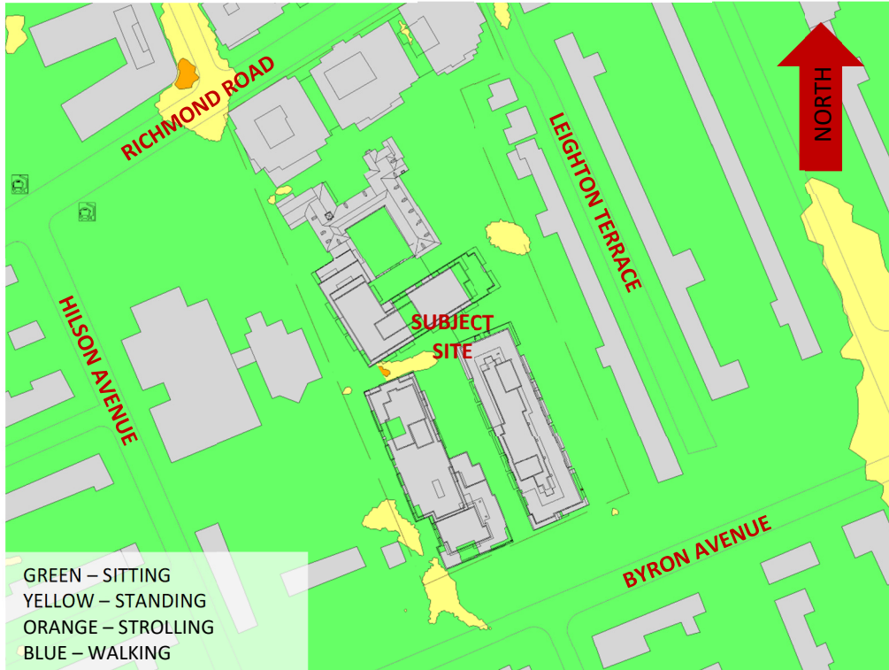
FIGURE 3A: SPRING – WIND CONDITIONS AT GRADE LEVEL
