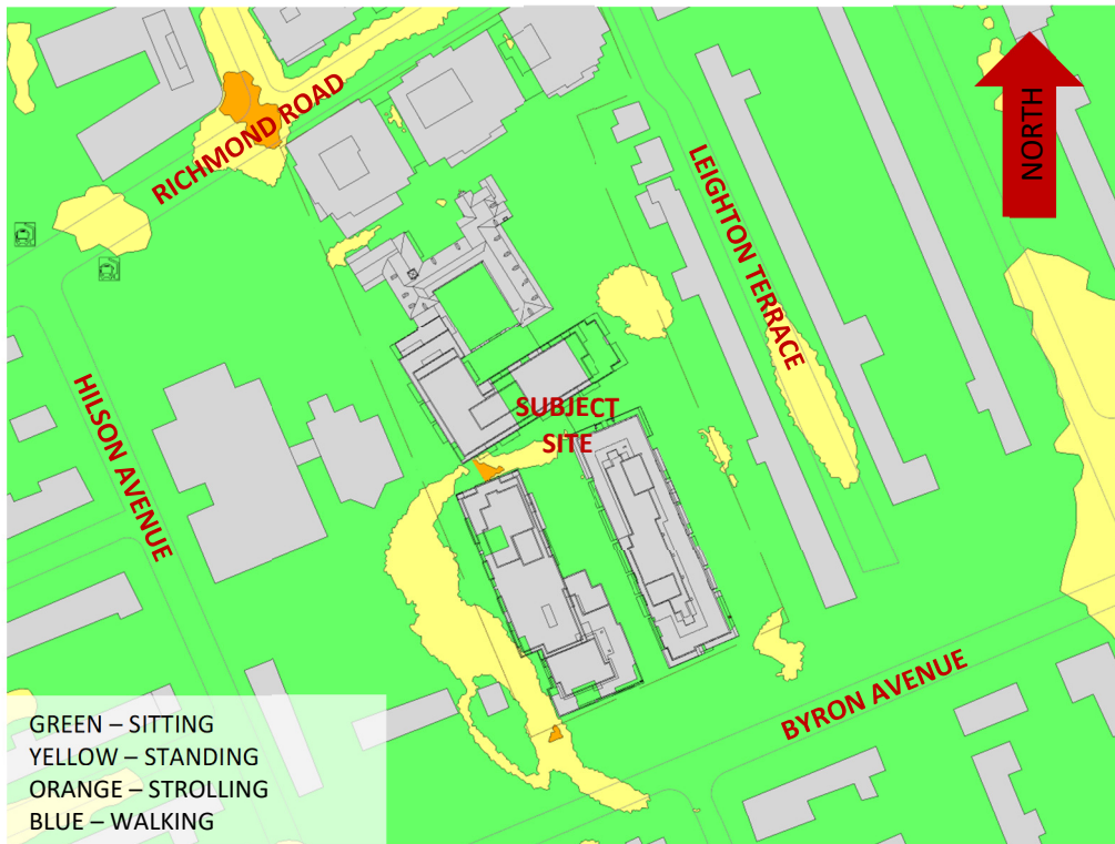
FIGURE 3D: WINTER – WIND CONDITIONS AT GRADE LEVEL
