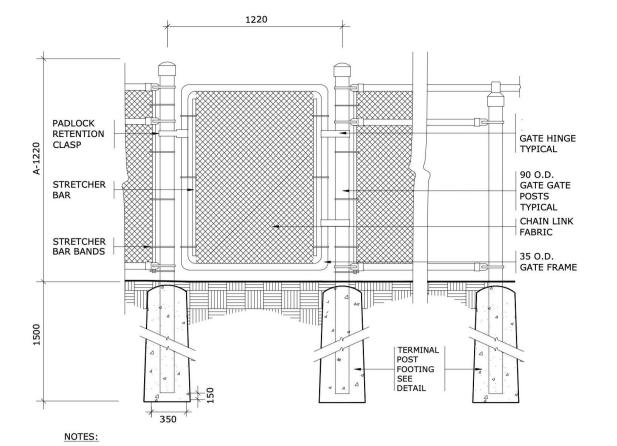
ALL MEASUREMENTS ARE IN MILLIMETRES UNLESS OTHERWISE NOTED GATE FRAMES SHALL BE CONSTRUCTED OF 33 O.D. GALVANIZED STEEL PIPE. SHOP BENT, WELDED
