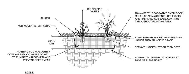
ALL MEASUREMENTS IN MILLIMETERS UNLESS OTHERWISE NOTED. LOCATION OF PERENNIAL BEDS SPECIFIED ON DRAWINGS L.1 - L.5. PLANTING SOIL MIX AS PER SPECIFICATIONS. 4. PROVIDE 100mm HIGH EARTH SAUCER AROUND PERENNIAL/GRASS BED
