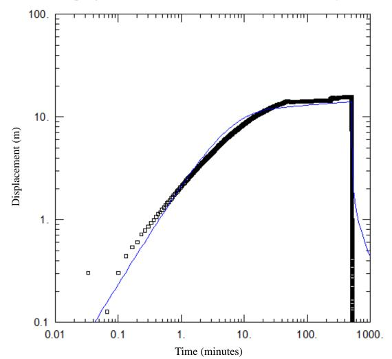
Transmissivity:  $5 \text{ m}^2/\text{day}$  ( $6 \text{ x } 10^{-5} \text{ m/s}$ )
