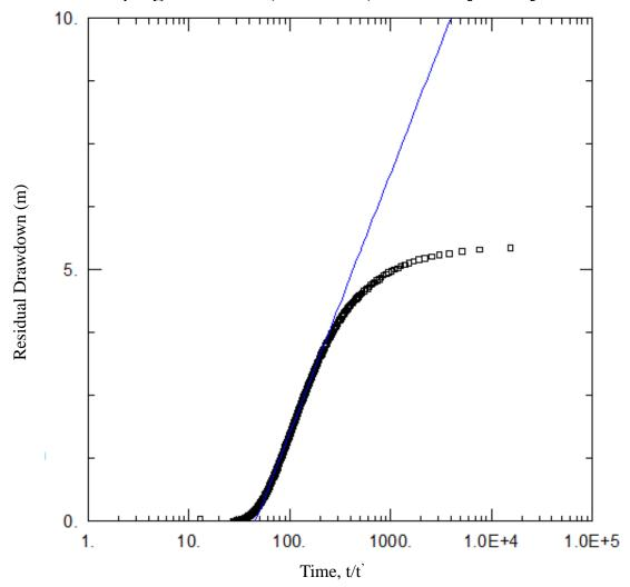
Transmissivity:  $2 \text{ m}^2/\text{day} (2 \text{ x } 10^{-5} \text{ m/s})$
