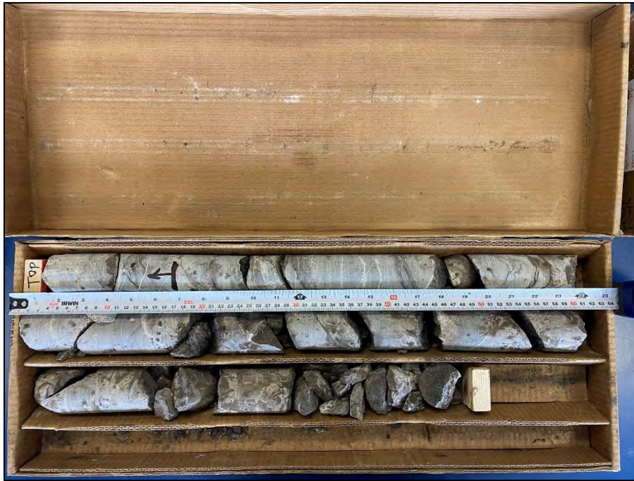
Photo 44: Photograph of RC 11 from BH 5-23 – Depth from 19.58 to 21.18 m – RQD = 52 % and REC = 100 %
