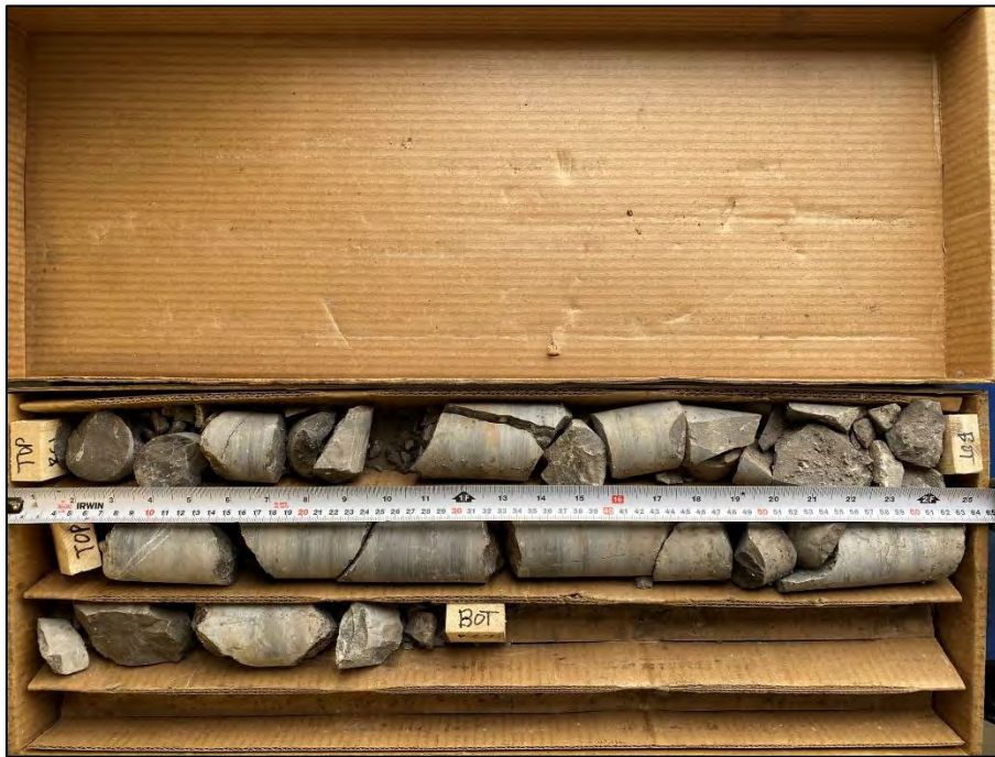
Photo 36: Photograph of RC 3 from BH 5-23 – Depth from 7.04 to 8.69 m – RQD = 49 % and REC = 100 %
