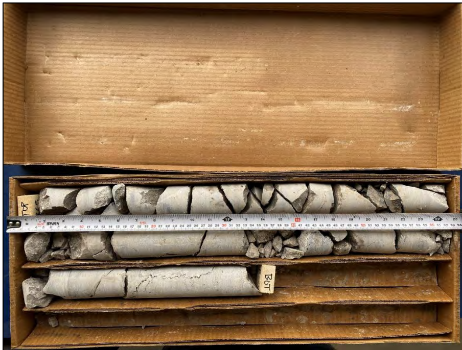
Photo 38: Photograph of RC 5 from BH 5-23 – Depth from 10.13 to 11.63 m – RQD = 32 % and REC = 100 %
