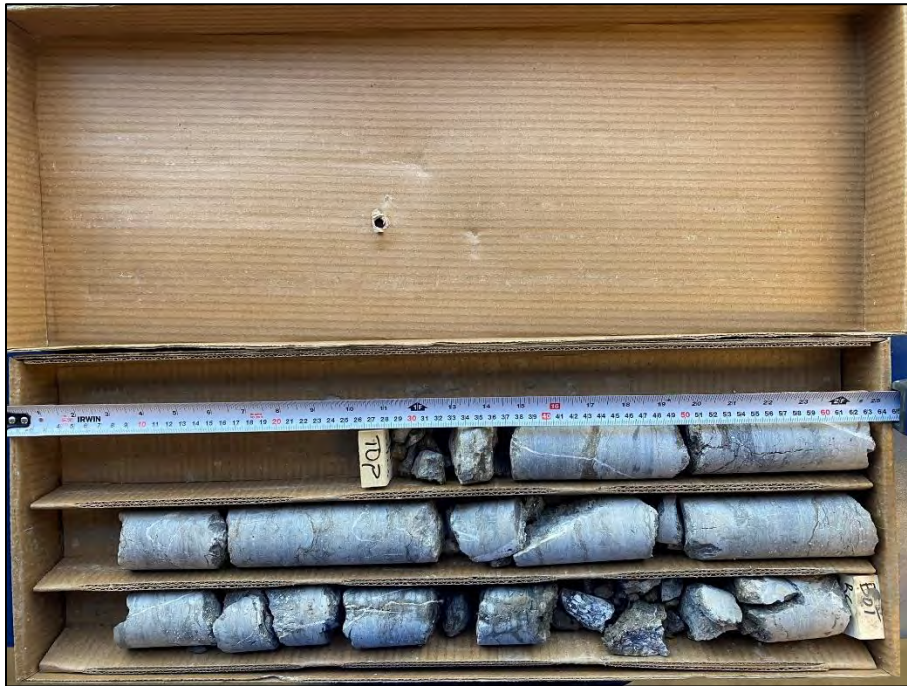
Photo 22: Photograph of RC 11 from BH 2-23 – Depth from 16.69 to 18.16 m – RQD = 41 % and REC = 98 %
