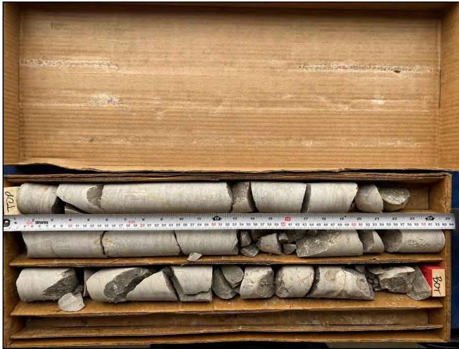
Photo 38: Photograph of RC 5 from BH 5-23 – Depth from 10.13 to 11.63 m – RQD = 32 % and REC = 100 %
