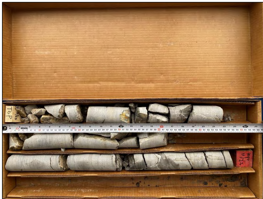
Photo 4: Photograph of RC 4 from BH 1-23 – Depth from 6.15 to 7.65 m – RQD = 59 % and REC = 100 %
