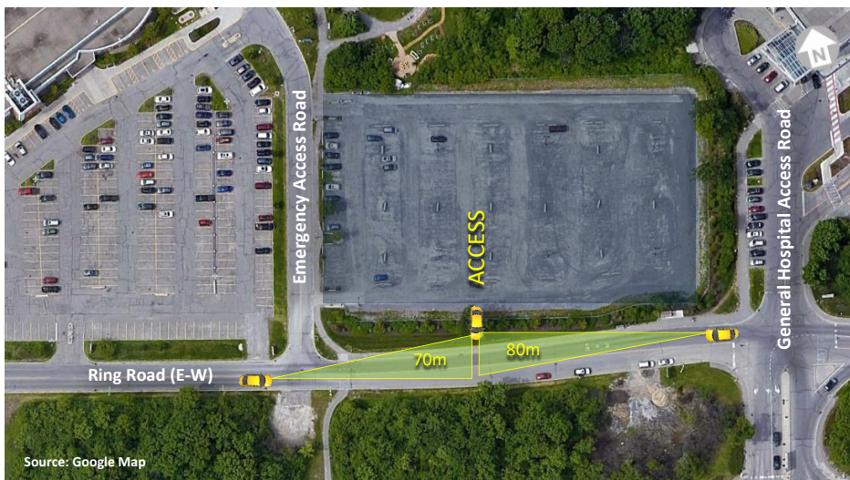
Figure 11: Ring Road (E-W) Access Intersection Sight Distance
