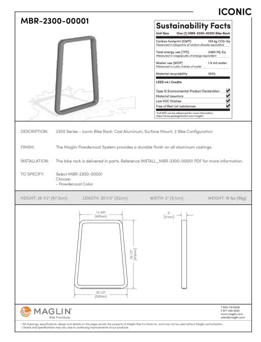
COLOUR: SILVER 14 SURFACE MOUNT TO CONCRETE PAVING WITH STAINLESS STEEL, TAMPER PROOF HARDWARE
