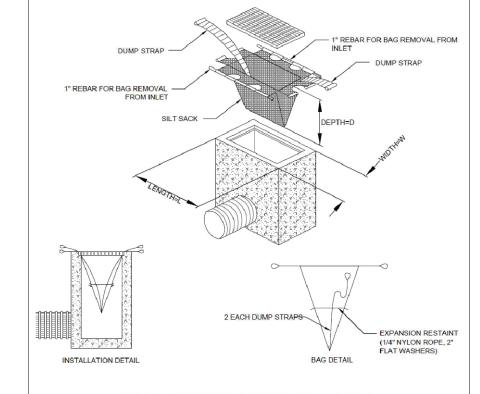
INLET SEDIMENT CONTROL DEVICE
