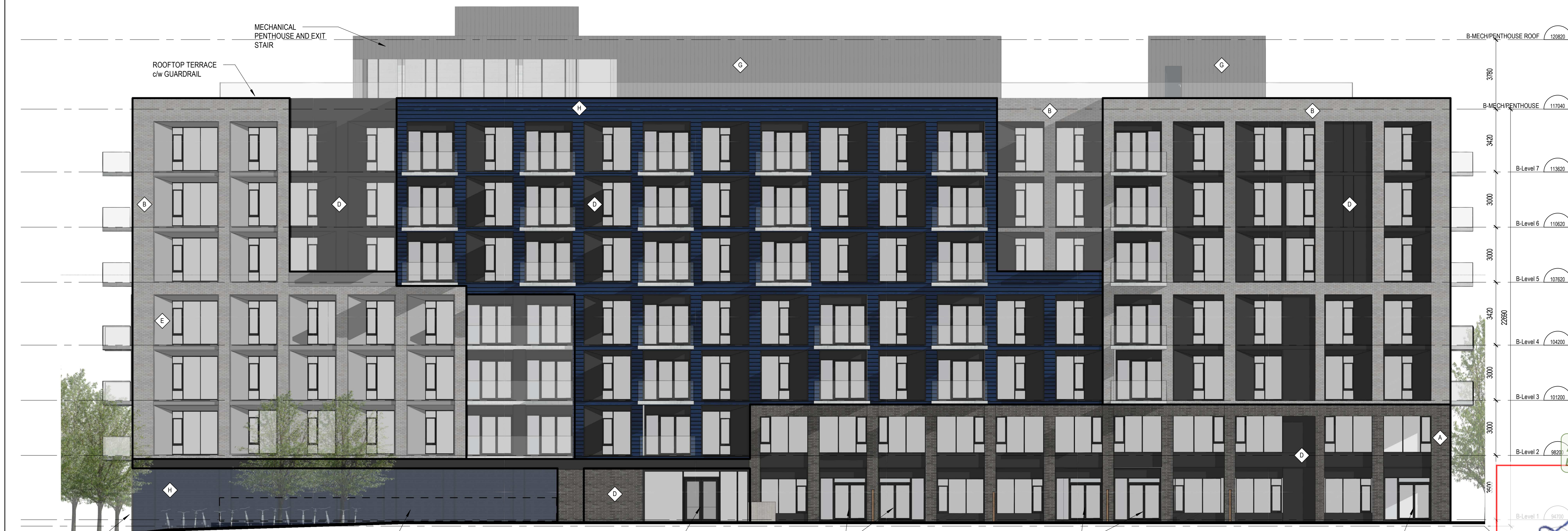
2 BLDG B NORTH ELEVATION ÉCHELLE / SCALE: 1:125
