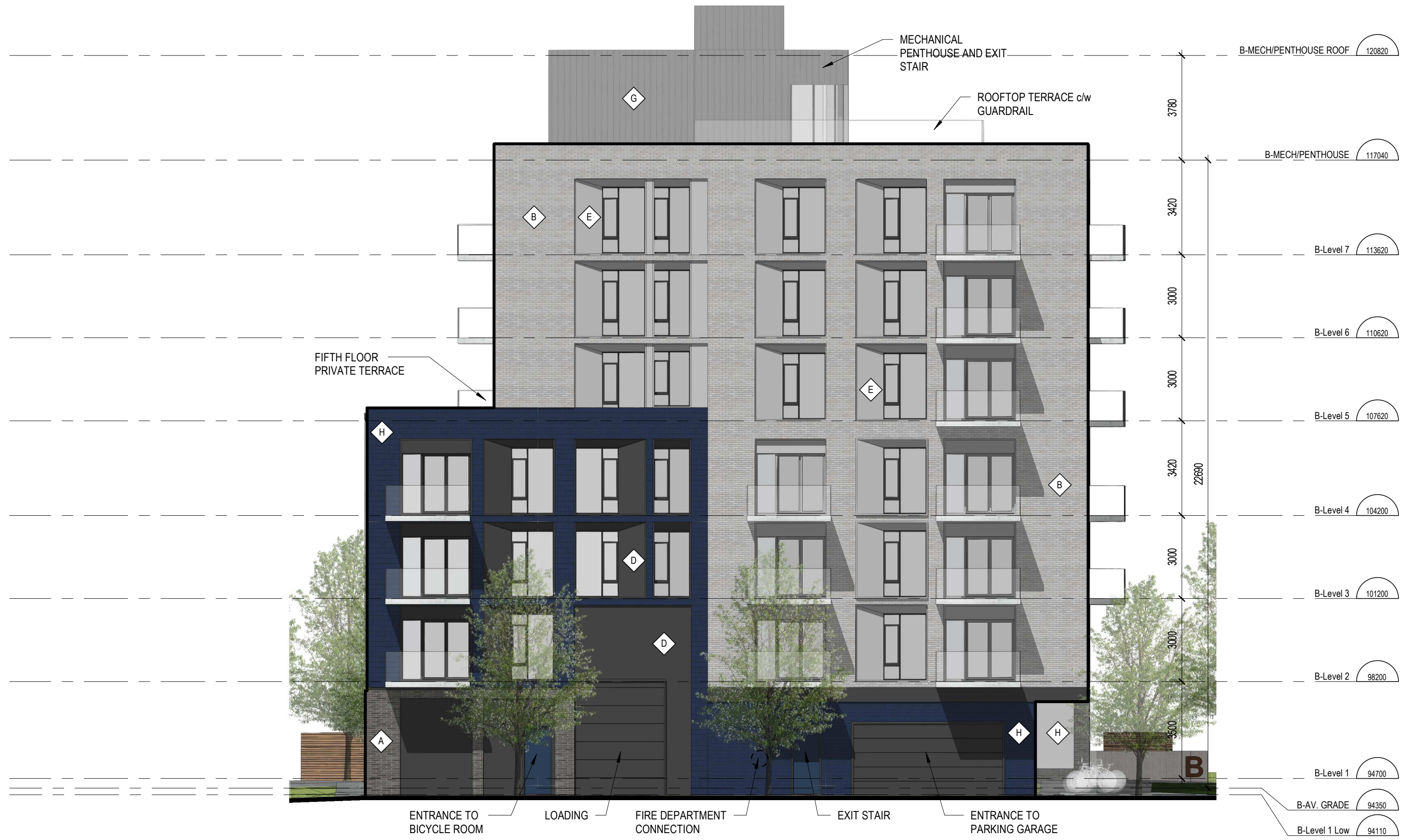
2 BLDG B EAST ELEVATION ÉCHELLE / SCALE: 1:125
