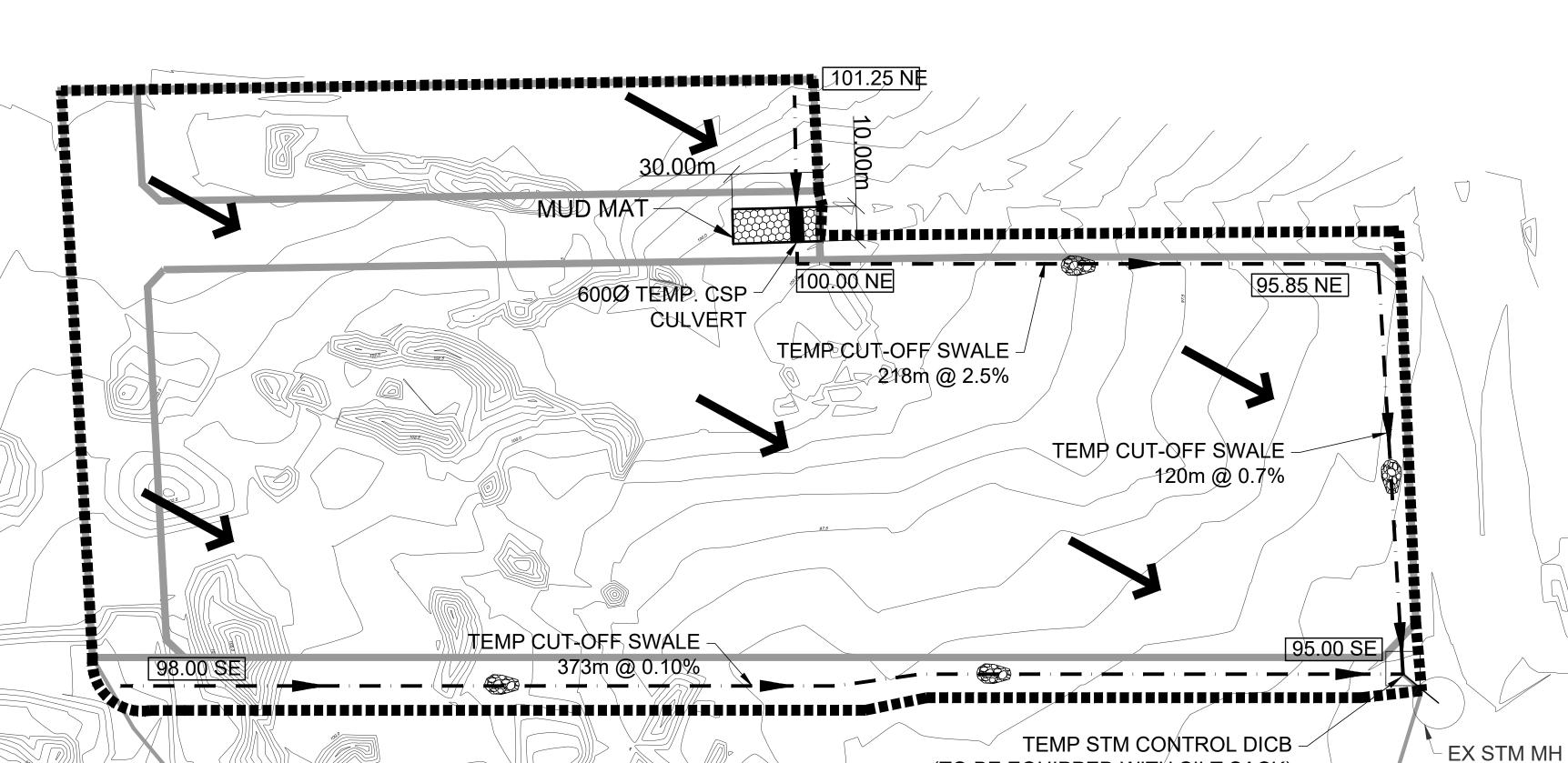
TEMP STM CONTROL DICB (TO BE EQUIPPED WITH SILT SACK)
