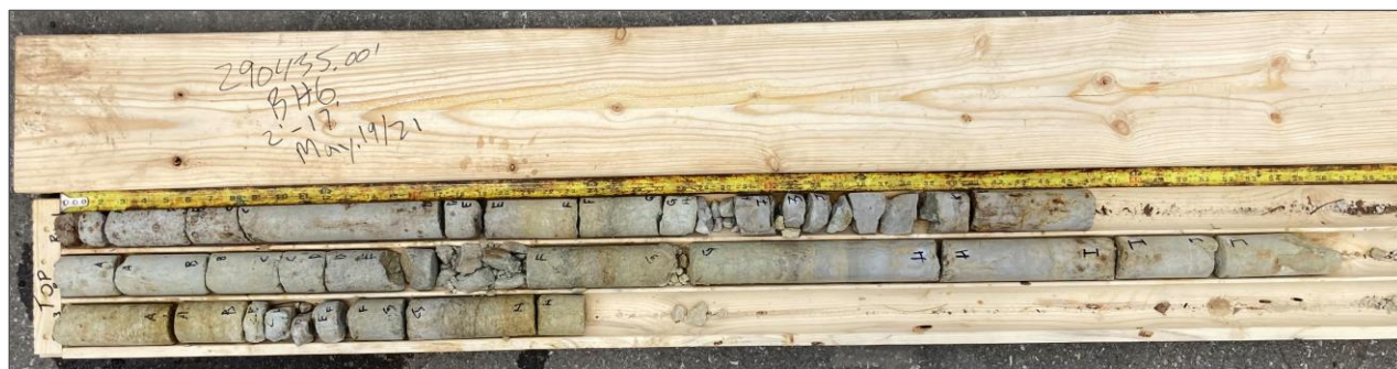
Photo 2 – Borehole BH6, Rock Core (Runs 1 to 3)
