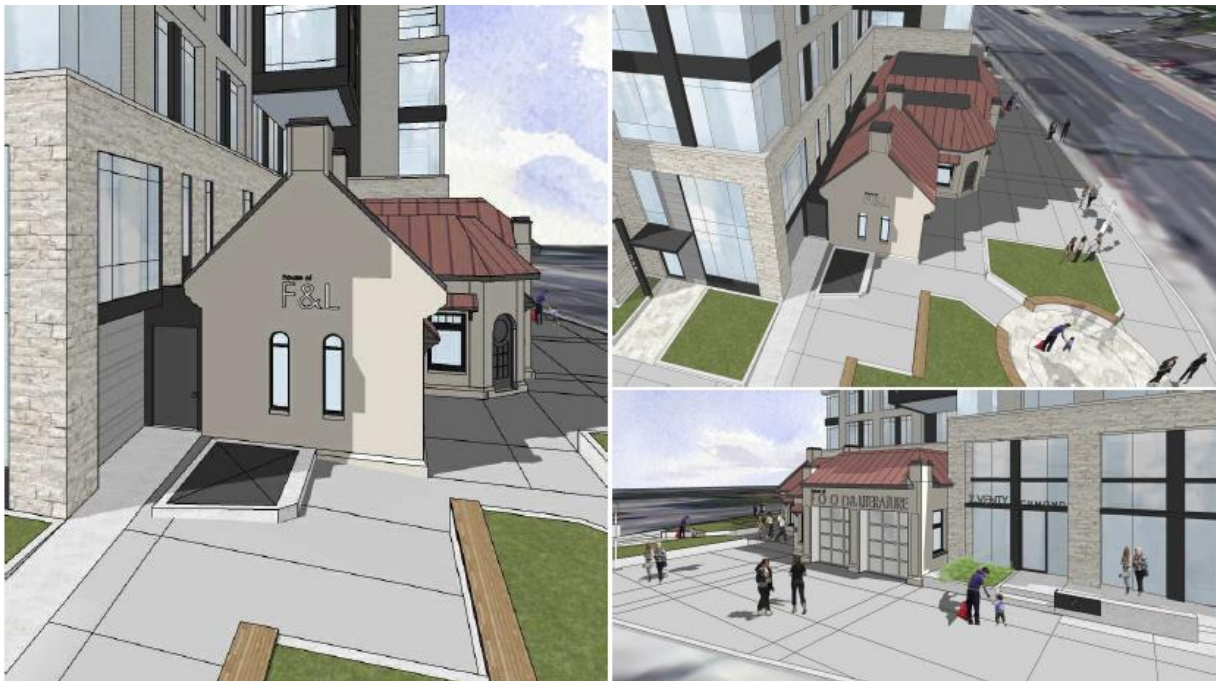
Figure 13: Views clockwise - 1. from the west illustrating the recessed link between the Station and the apartment, 2. Aerial view illustrating the massing and ability to interpret the entire building as a separate feature. 3. A view looking south east illustrating the side window. Source: Hobin architecture 2023.
