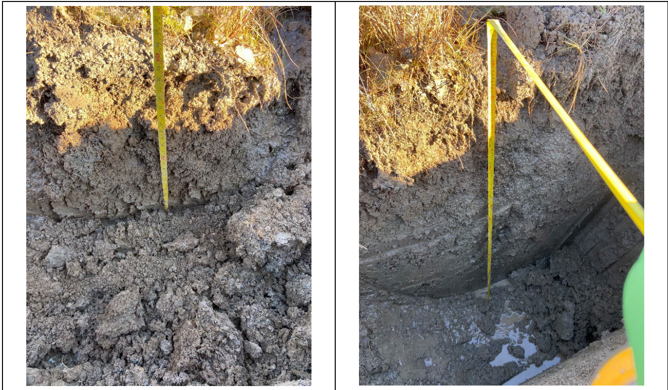
Sample SS-1 submitted for Reg 153 metals, OCP, HPA, CN, EC, SAR and pH analysis.
