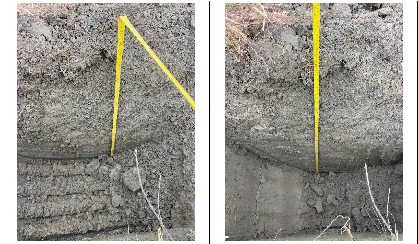
Sample SS-1 submitted for Reg 153 metals, CN, EC, SAR and pH analysis.
