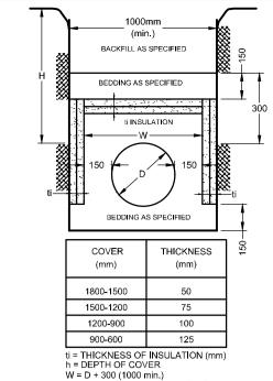
W = D + 300 (1000 min.) W = WIDTH OF INSULATION (mm) D = O.D OF PIPE (mm)
