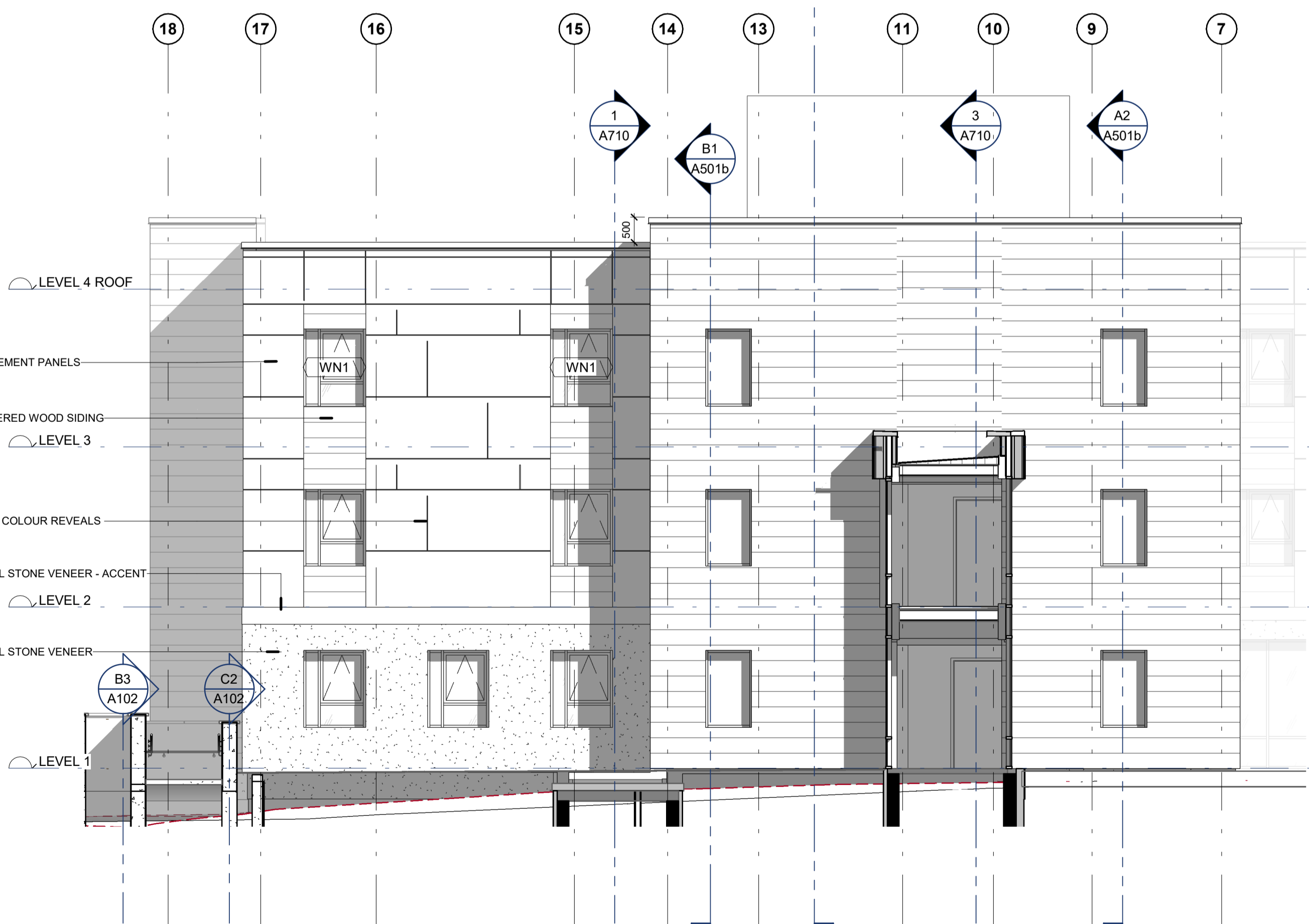
A5 ELEVATION - BLDG B - SOUTH, WEST A401b 1:75
