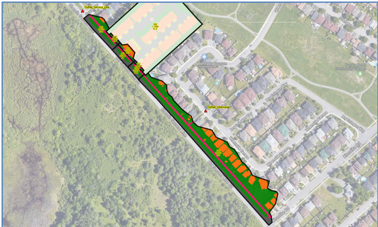
Figure 1 – Subcatchments Used for Sizing Entrance Culverts
