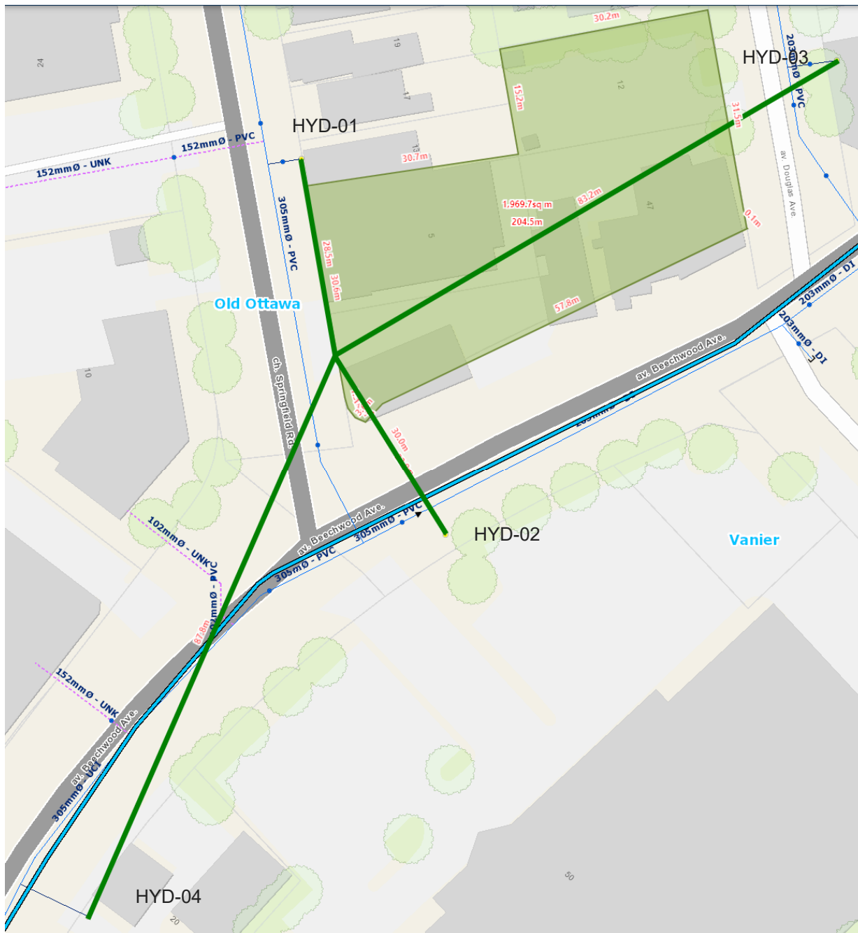
Figure 3-1: Fire Hydrant Coverage Sketch
