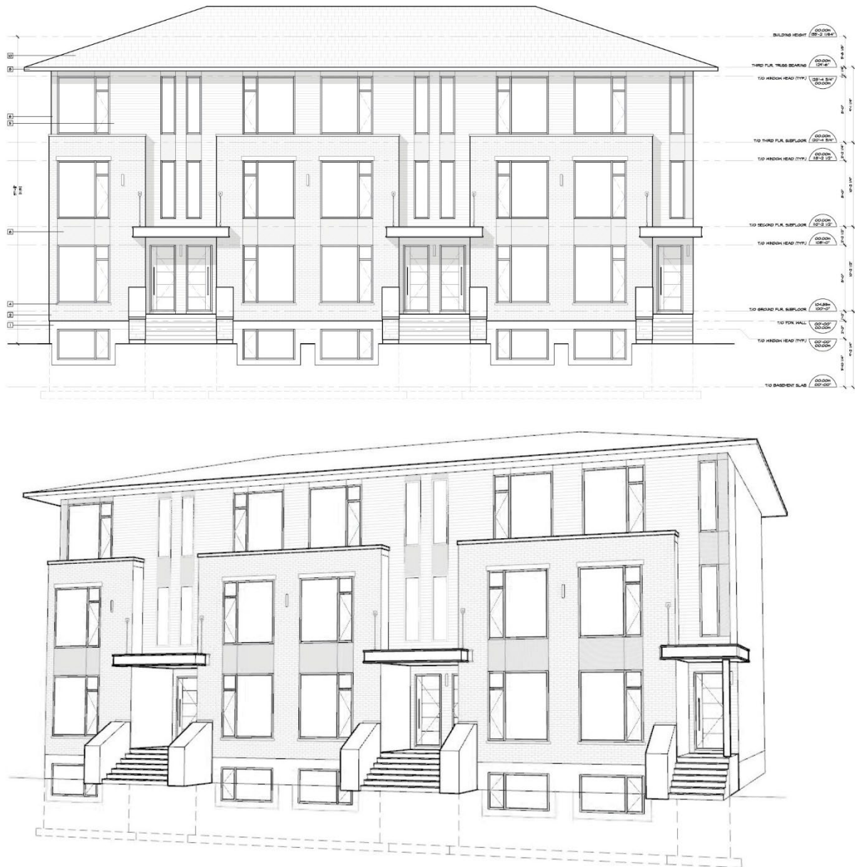
Figure 8: Elevation and Perspective drawing of the proposed 10 unit stacked townhouse dwelling type.
