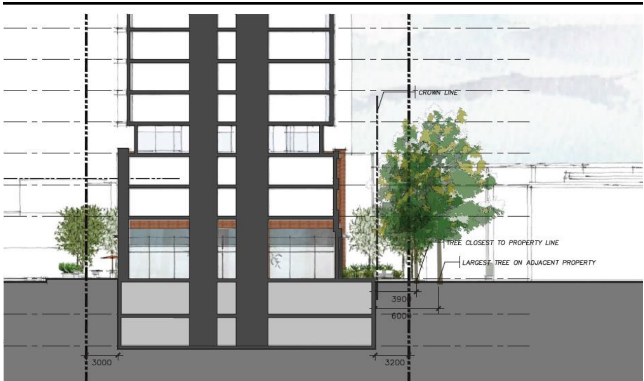
Figure 22: a cross-section of the proposed building illustrating property lines and setbacks from neighbouring properties. The underground parking is setback to avoid damaging the root system of existing mature trees. Hobin Architecture 2020.
