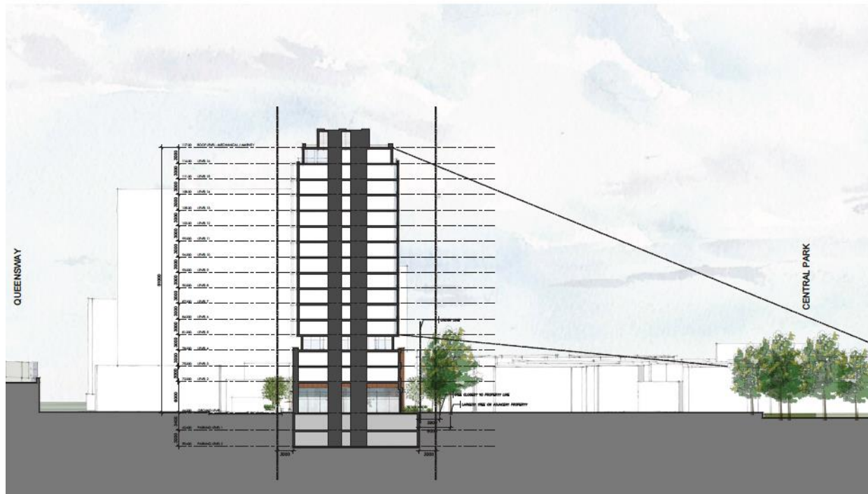
Figure 14: The section through the proposed development illustrates the view plan from Central Park. Because of the grade changes and the extensive buffer from trees, views of the tower are filtered. Source Hobin Architecture 2020.
