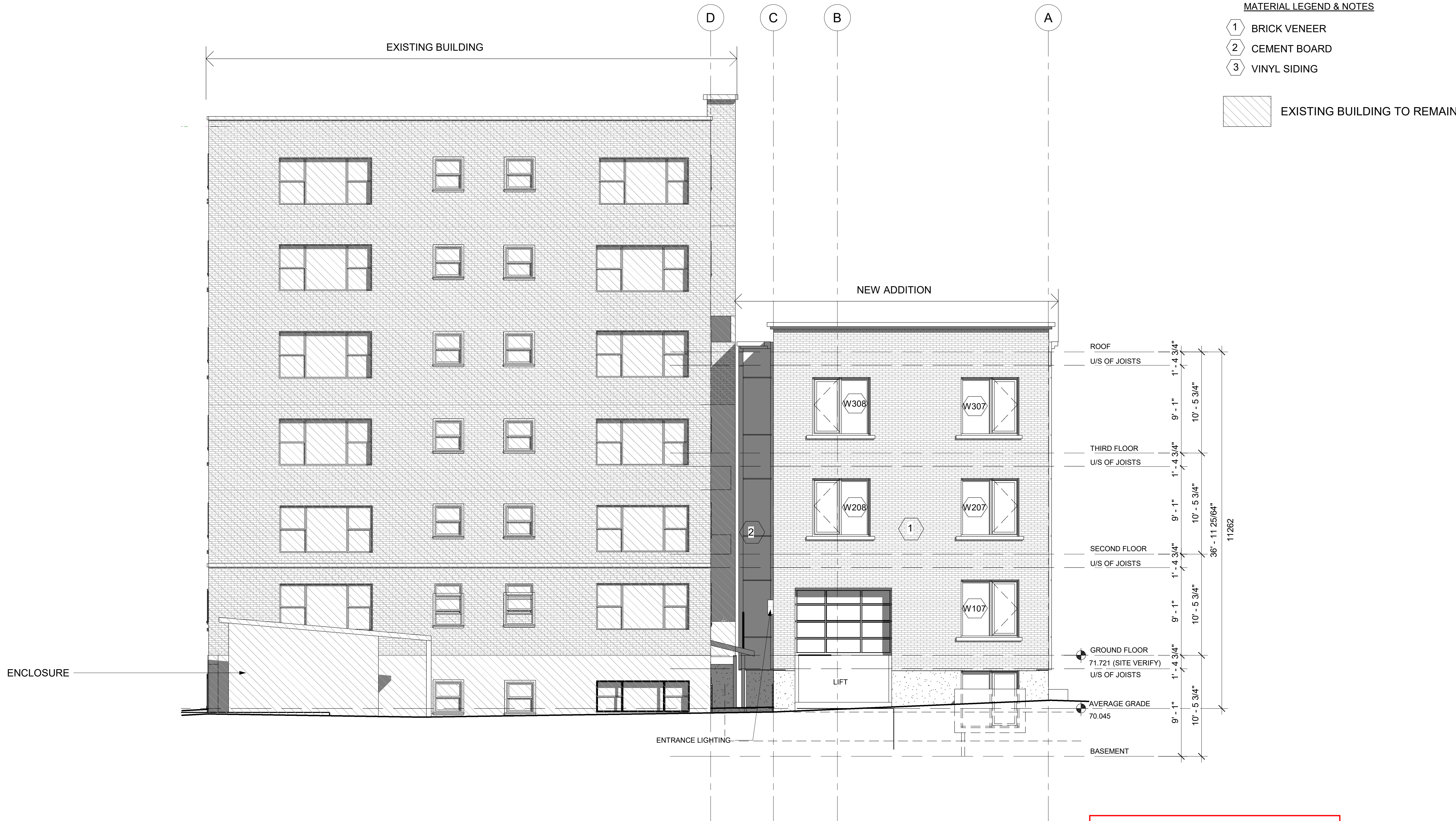
1 Rear ( South) Elevation 3/16" = 1'-0"
