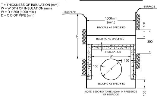
NOTE: BEDDING TO BE 300mm IN PRESENCE OF BEDROCK **INSULATION DETAIL FOR SHALLOW SEWERS & WATERMAIN**
