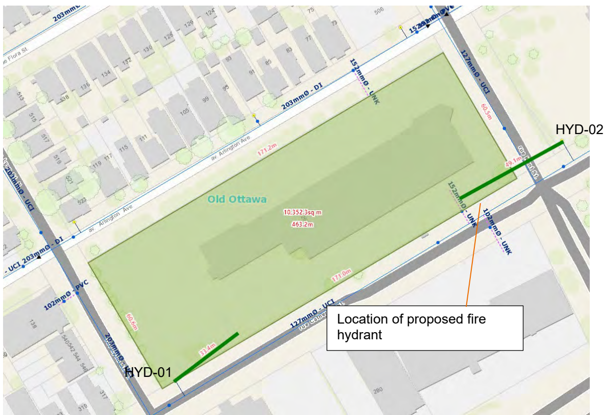
Figure 3-1: Fire Hydrant Coverage Sketch
