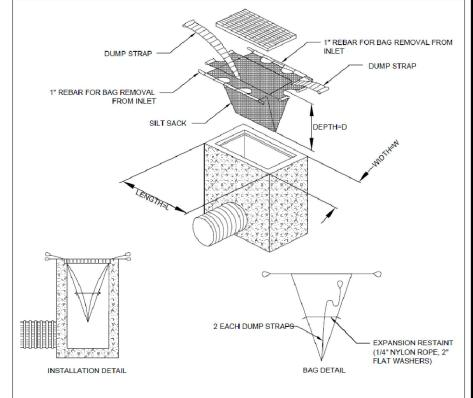
INLET SEDIMENT CONTROL DEVICE
