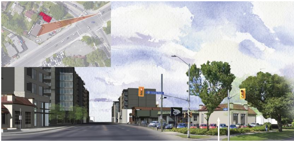
Figure 8: Plan and view illustrating the temporary location for storing the Service Station across from the Richmond Road site. In its temporary location the hydraulic wheels will be removed and the building set on cribbing.
