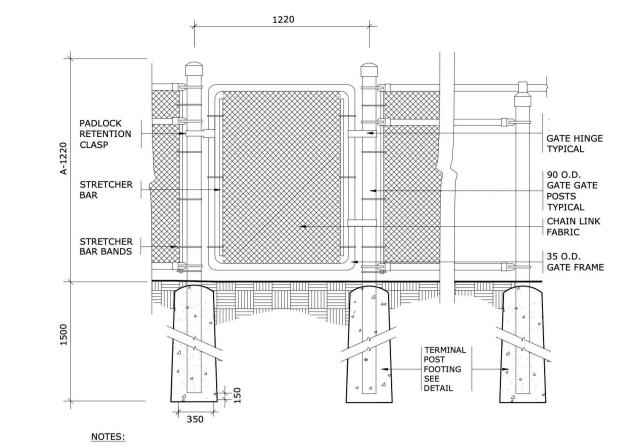
ALL MEASUREMENTS ARE IN MILLIMETRES UNLESS OTHERWISE NOTED GATE FRAMES SHALL BE CONSTRUCTED OF 33 O.D. GALVANIZED STEEL PIPE. SHOP BENT, WELDED
