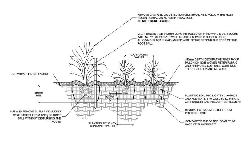
ALL MEASUREMENTS IN MILLIMETERS UNLESS OTHERWISE NOTED. LOCATION OF SHRUBS SPECIFIED ON DRAWINGS L.1 - L.5. PLANTING SOIL MIX AS PER SPECIFICATIONS PROVIDE 100mm HIGH EARTH SAUCER AROUND SHRUBS STAKE SHRUBS LARGER THAN 1500mm TALL AT TIME OF PLANTING. 6. STAKES TO BE REMOVED AT THE END OF THE WARRANTY PERIOD
