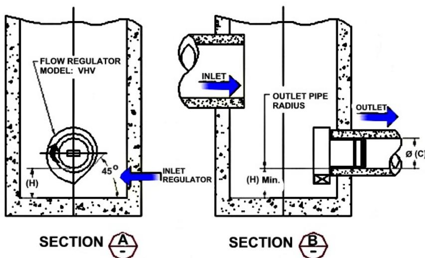
**FLOW REGULATOR TYPICAL INSTALLATION IN SQUARE MANHOLE**
