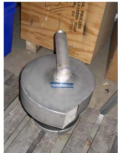
**VHV with air vent for minimal slopes**
