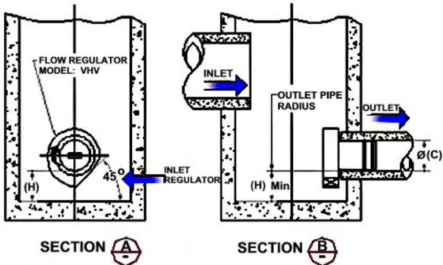
**FLOW REGULATOR TYPICAL INSTALLATION IN CIRCULAR MANHOLE**
