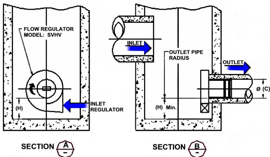
**FLOW REGULATOR TYPICAL INSTALLATION IN SQUARE MANHOLE**
