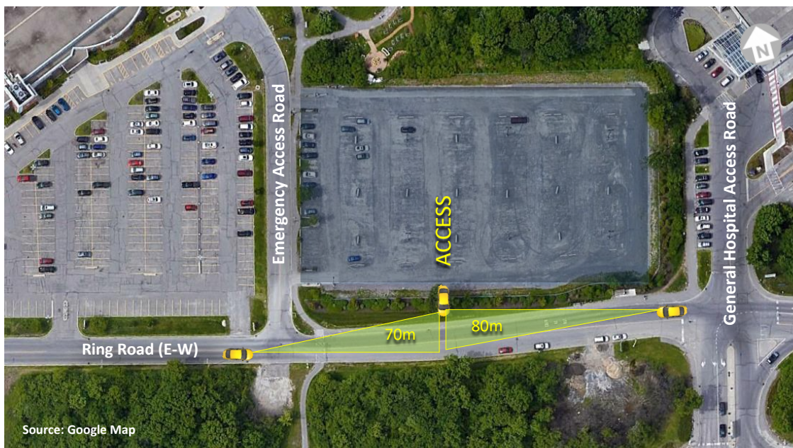
Figure 11: Ring Road (E-W) Access Intersection Sight Distance
