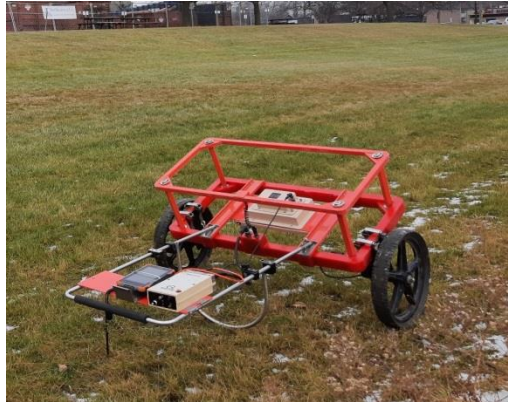
Figure 3-2: Typical TDEM Acquisition System Setup
