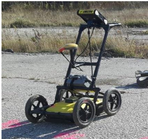
Figure 3-3: Typical GPR 250MHz Smart Cart System Setup
