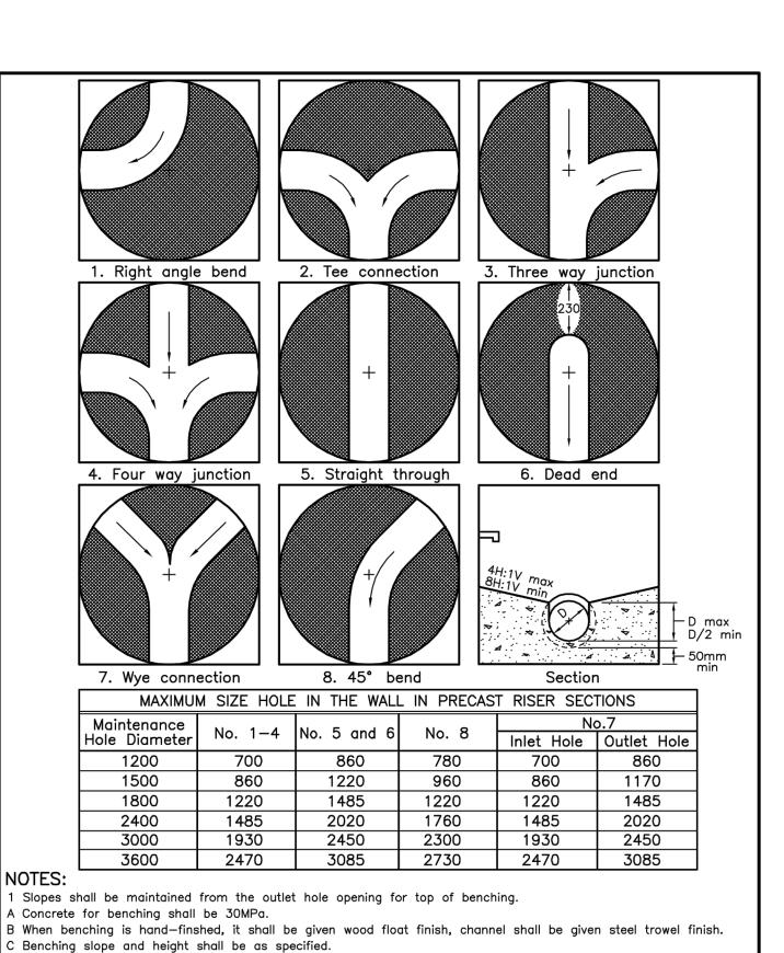
D When specified, maintenance holes that are 1200mm in diameter with a uniform channel for 200 or 250mm pipe may be prebenched at the manufacturer with standardized benching slope and channel orientation.
