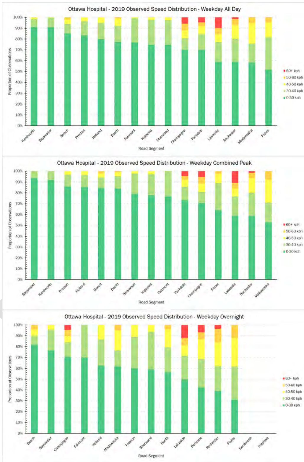
Figure 2: Summary of Weekday Vehicle Speed Distributions by Time of Day for Key Study Area Road Segments
