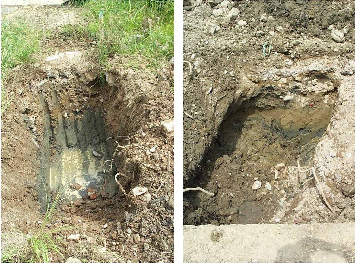
FIG. 4-27: Photographs of test pits for vane shear tests VST-3 and 4 that show the characteristics of the surface fill and underlying fine-grained soils. (source: [http://peer.berkeley.edu/lifelines/research\\_projects/3A02/](http://peer.berkeley.edu/lifelines/research_projects/3A02/))
