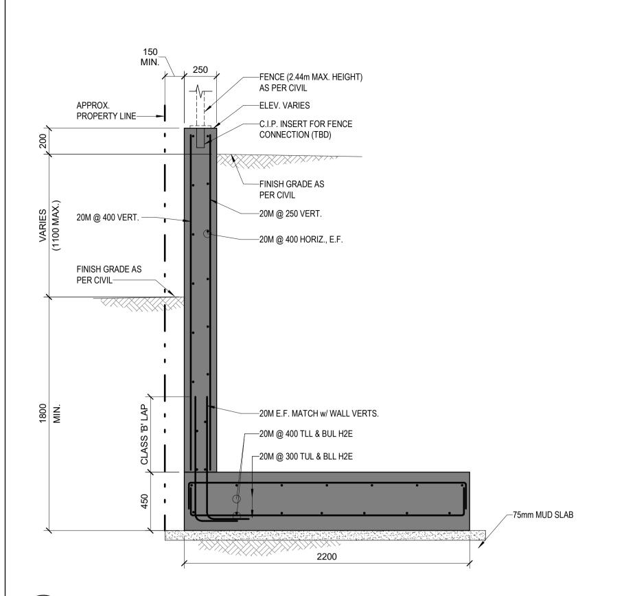
FENCE (2.44m MAX. HEIGHT) AS PER CIVIL -ELEV. VARIES —C.I.P. INSERT FOR FENCE CONNECTION (TBD) \_\_\_\_20M @ 250 VERT. 20M @ 400 VERT.-—20M @ 400 HORIZ., E.F. FINISH GRADE AS PER CIVIL-—20M E.F. MATCH w/ WALL VERTS. 500 —20M @ 300 TUL & BLL H2E -20M @ 400 TLL & BUL H2E -75mm MUD SLAB
