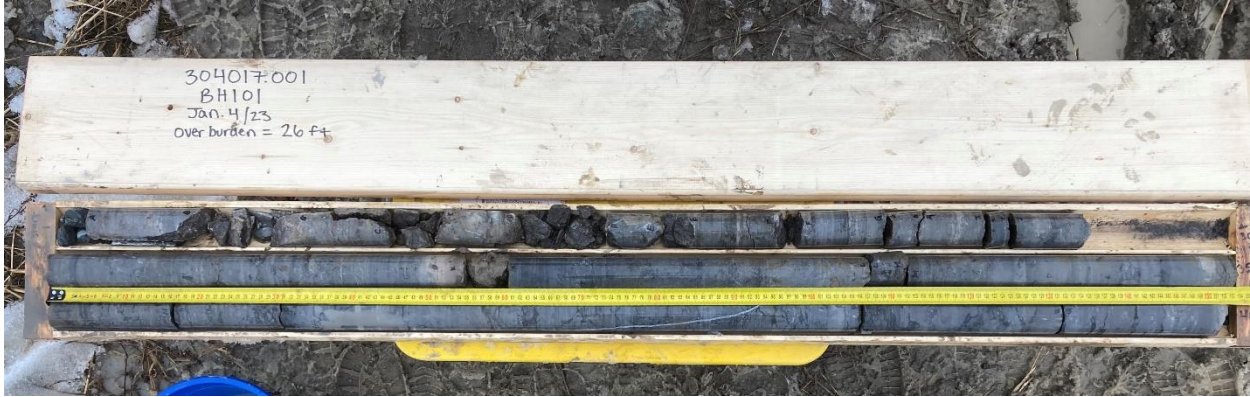
Photo 1 – Borehole BH101, Rock Core
