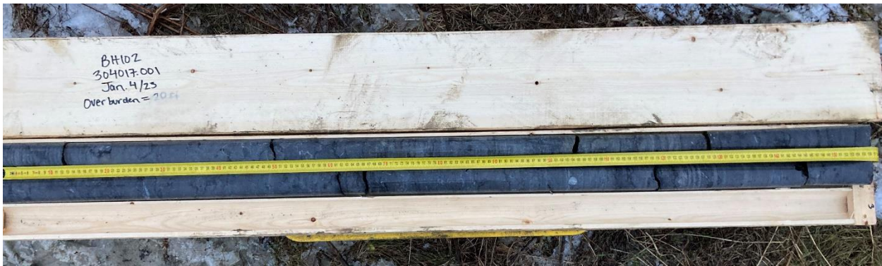
Photo 2 – Borehole BH102, Rock Core
