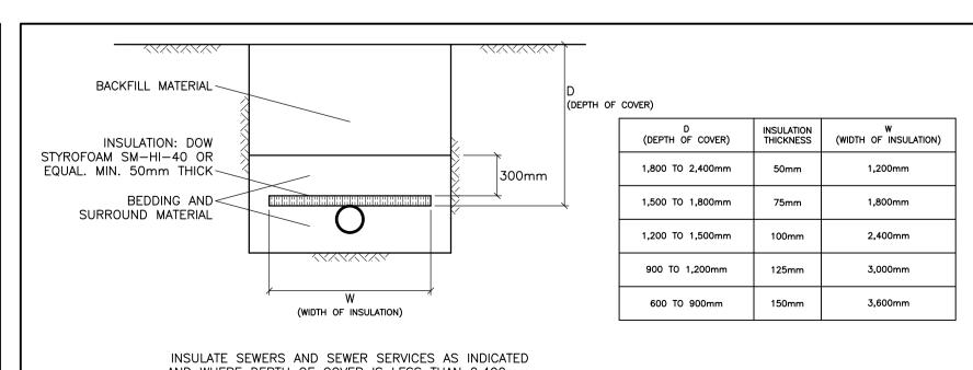
INSULATE SEWERS AND SEWER SERVICES AS INDICATED AND WHERE DEPTH OF COVER IS LESS THAN 2,400mm.
