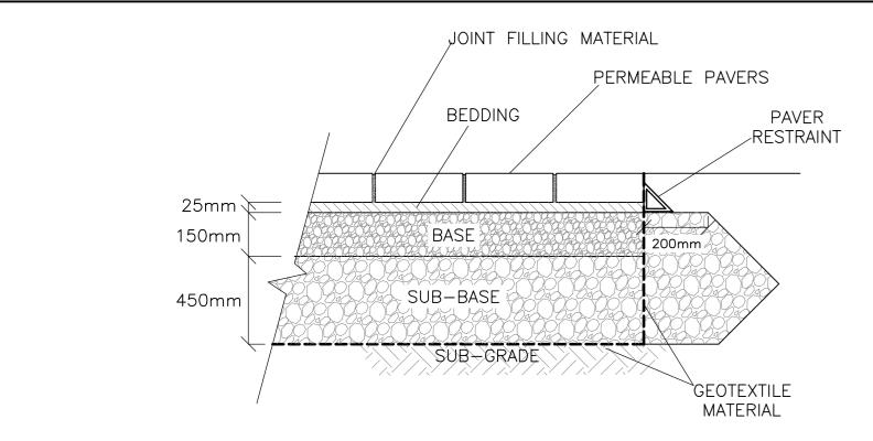
JOINT FILLING MATERIAL: 2.5-10mm AGGREGATE OR AS RECOMMENDED BY MANUFACTURER BEDDING COURSE: 2.5-10mm AGGREGATE OR AS RECOMMENDED BY MANUFACTURER BASE COURSE: 5-28mm AGGREGATE OR AS RECOMMENDED BY MANUFACTURER SUB-BASE COURSE: 40-80mm AGGREGATE OR AS RECOMMENDED BY MANUFACTURER COMPACT EACH LAYER AS RECOMMENDED BY MANUFACTURER
