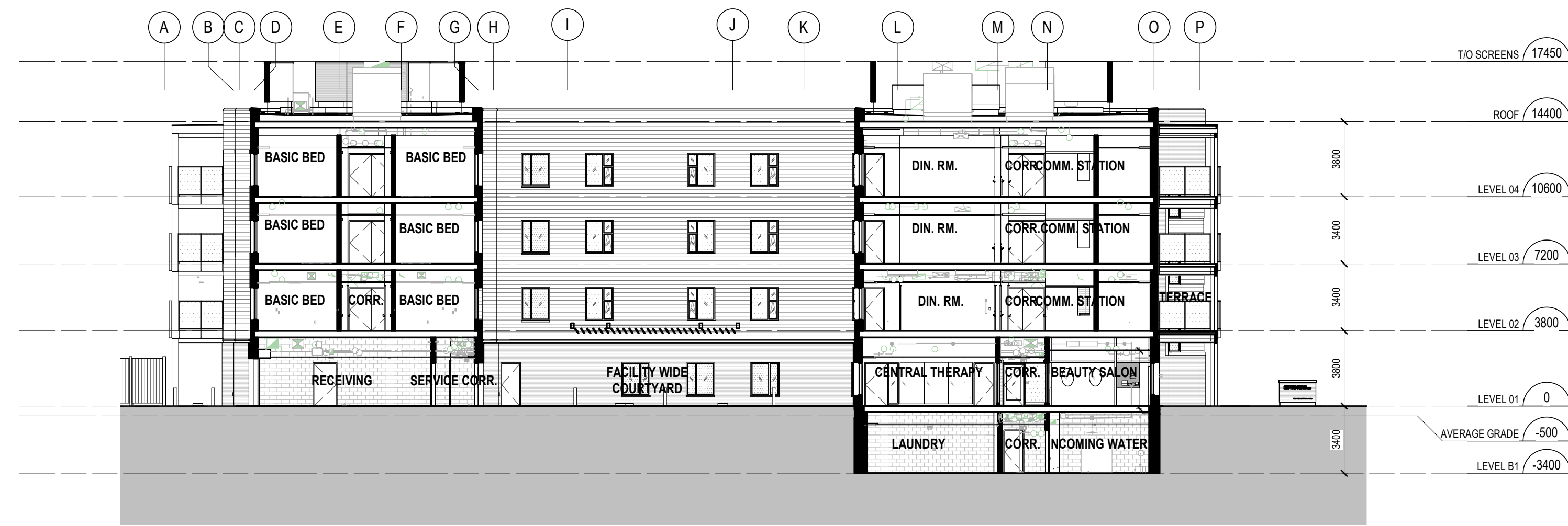
3 BUILDING SECTION - LOOKING NORTH A5.01 1:200
