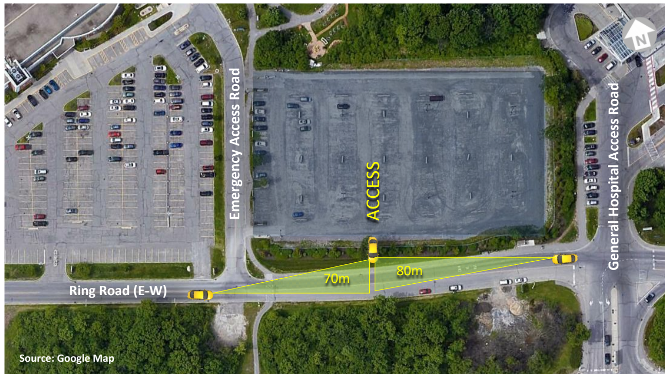
Figure 10: Ring Road (E-W) Access Intersection Sight Distance
