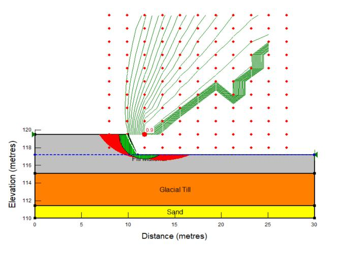
Name: Fill Material Model: Mohr-Coulomb Unit Weight: 18 kN/m<sup>3</sup> Cohesion: 0 kPa
