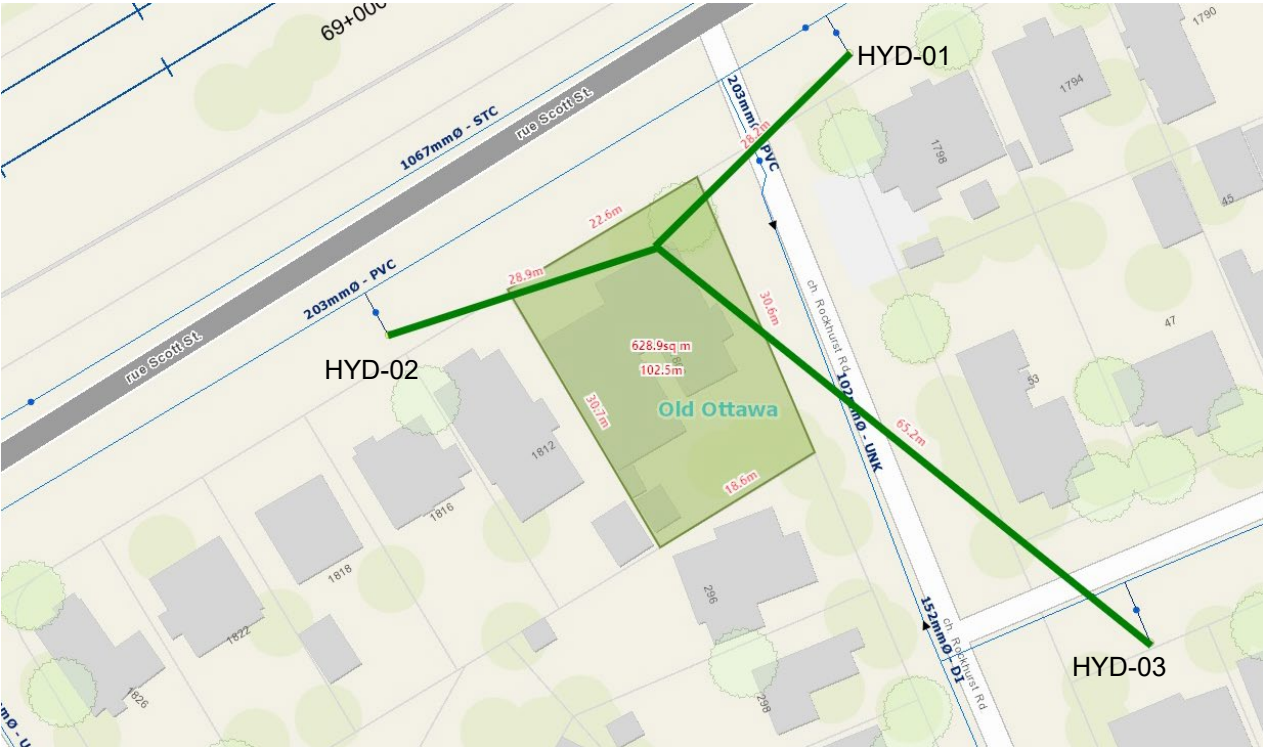
Figure 2: Fire Hydrant Coverage Sketch
