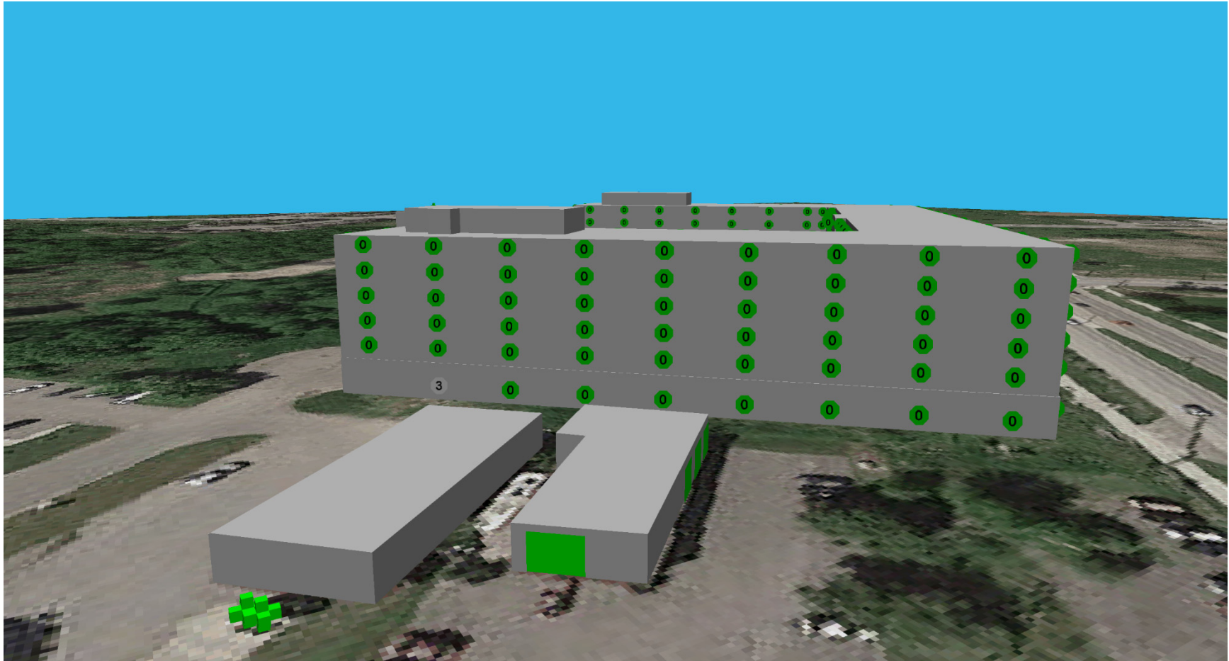
Figure 6b: Stationary Noise Excesses at Southwest Façade, Evening, Leq [dBA]
