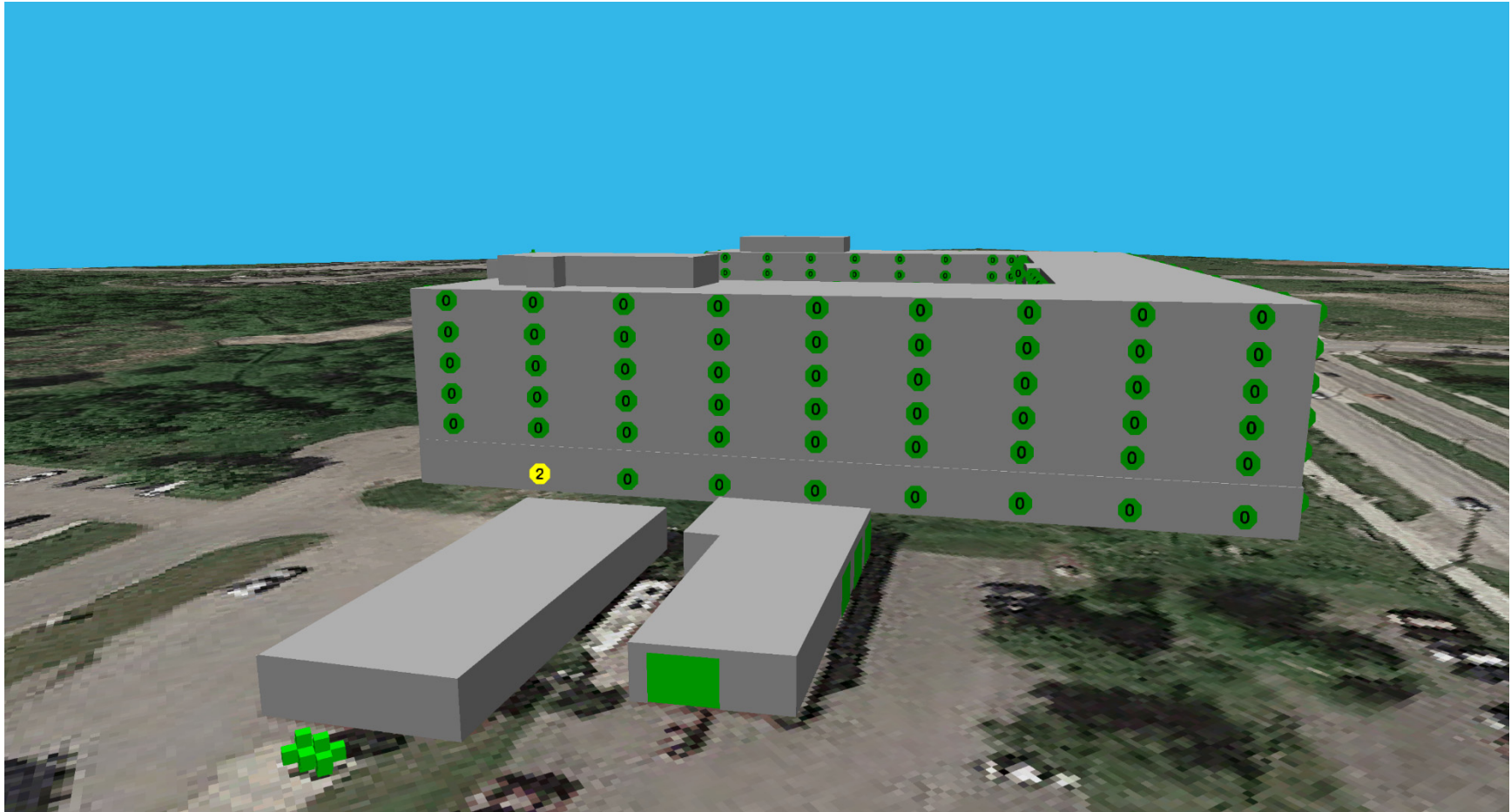
Figure 6a: Stationary Noise Excesses at Southwest Façade, Daytime, Leq [dBA]
