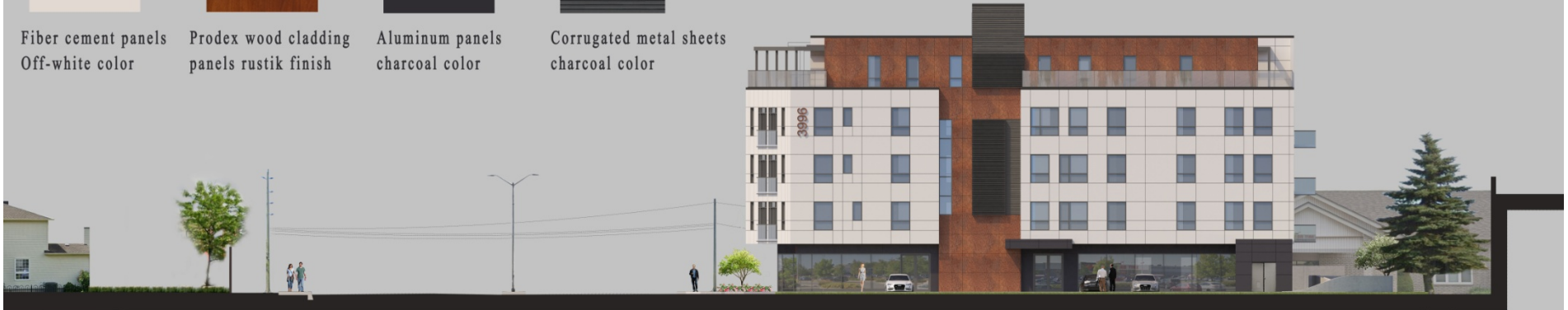
SOUTH WEST ELEVATION
