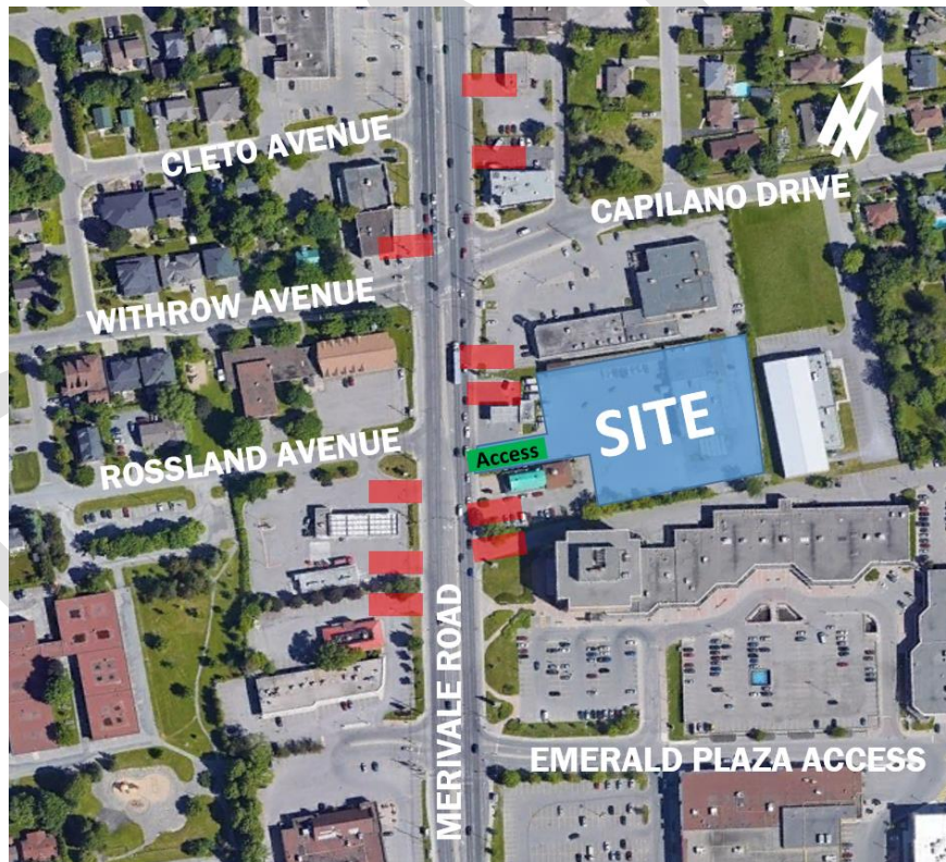
Figure 3: Adjacent Driveways within 200m of Site Access
