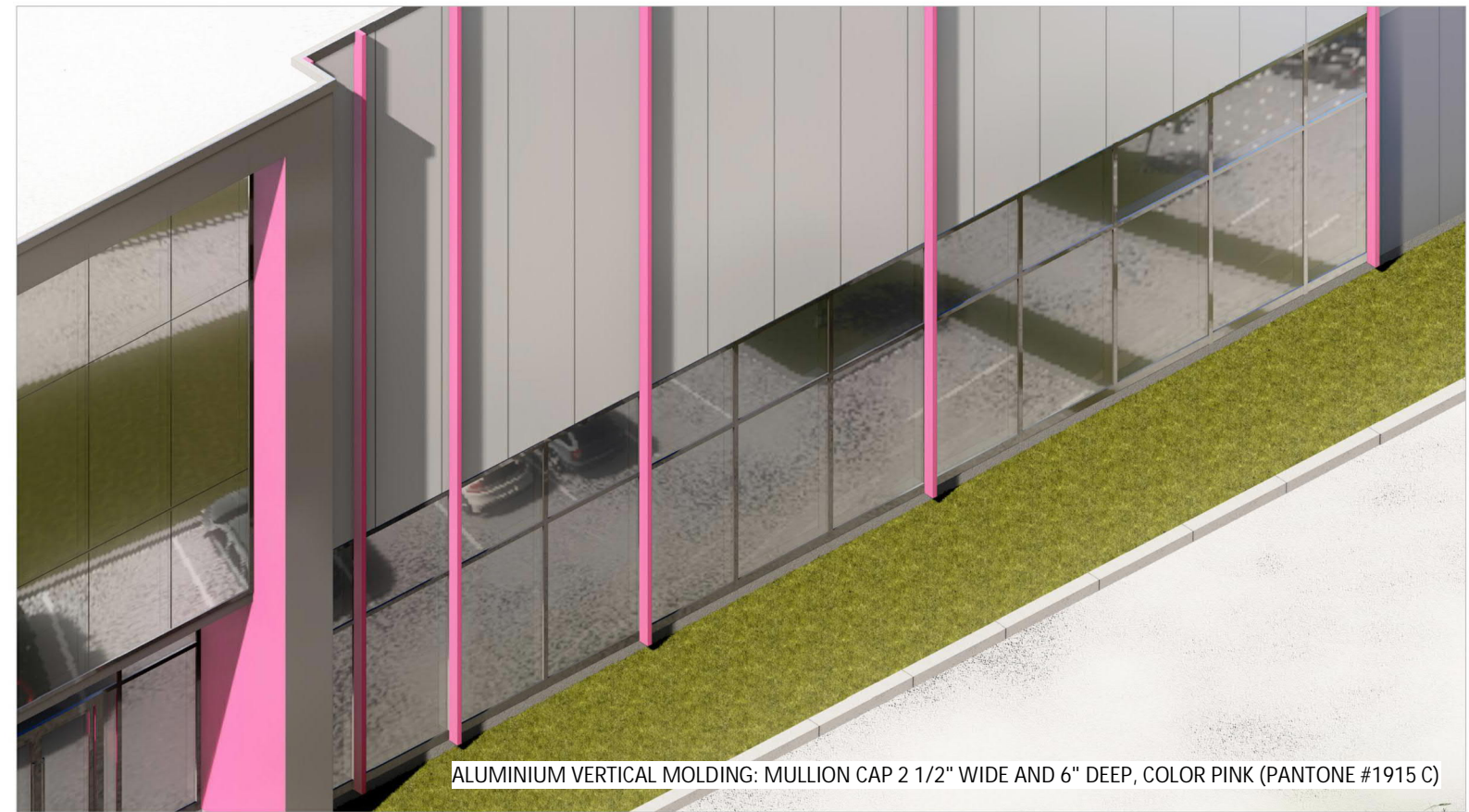
VERTICAL INSULATED METAL PANEL (IMP V.), 42" WIDE, 3" THICK, MICRO-RIB FINISH, COLOR: ZINC GRAY (REF. KINGSPAN)
