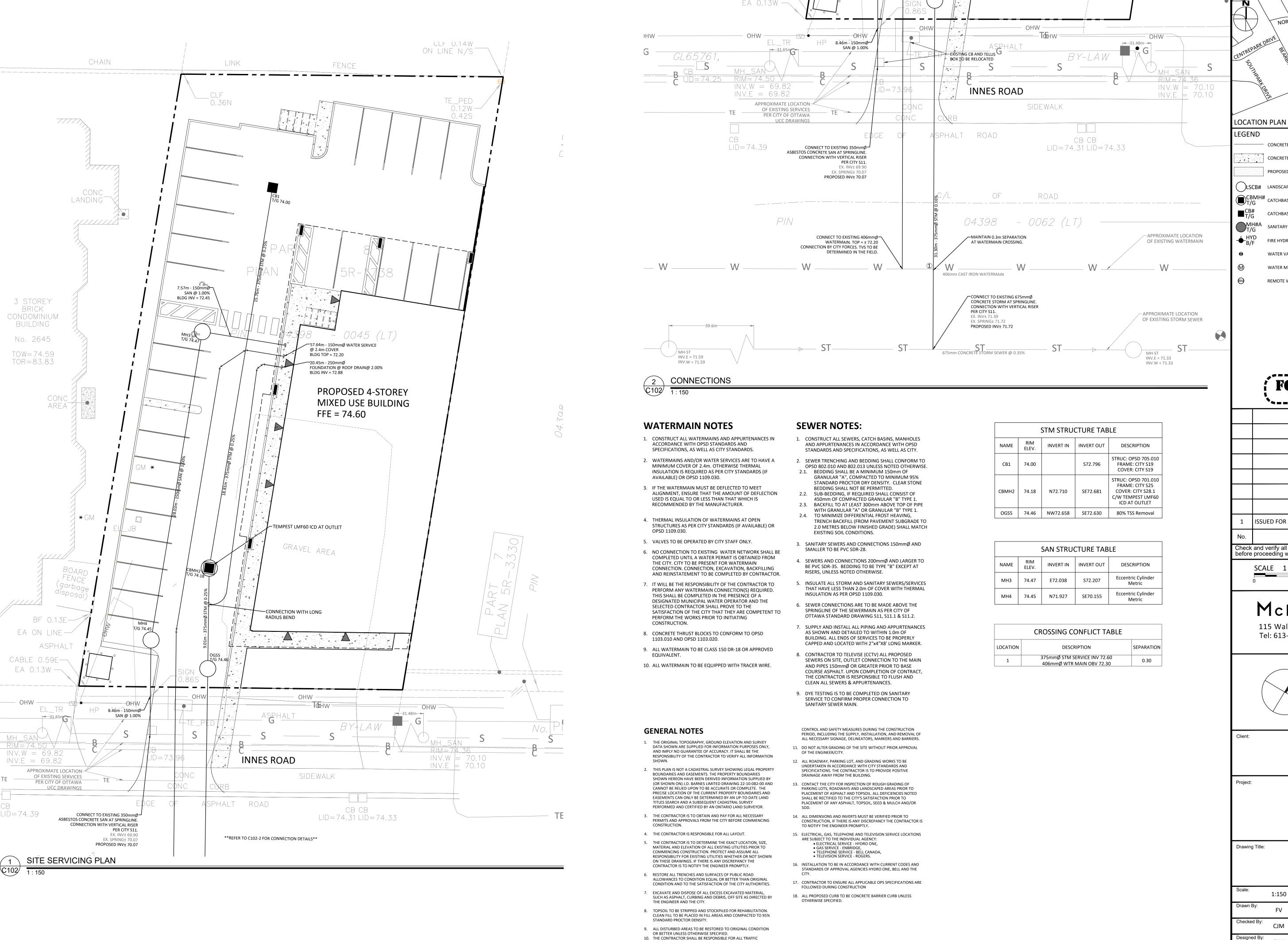
∕-SUBJECT SITE LIMIT OF CONSTRUCTION CONCRETE BARRIER CURB ----- DRAINAGE SWALE CONCRETE WALKWAY PROPOSED ASPHALT — · · · — DRAINAGE DITCH )LSCB# LANDSCAPING CATCHBASIN SURFACE ELEVATION CATCHBASIN MANHOLE SWALE ELEVATION TOP OF WALL ELEVATION BOTTOM OF WALL ELEVATION SANITARY SEWER MANHOLE OVERLAND FLOW ROUTE FIRE HYDRANT - SILT FENCE BARRIER WATER VALVE STRAW BALE CHECK DAM WATER METER MUD MAT REMOTE WATER METER NOT FOR CONSTRUCTION ISSUED FOR SITE PLAN CONTROL
