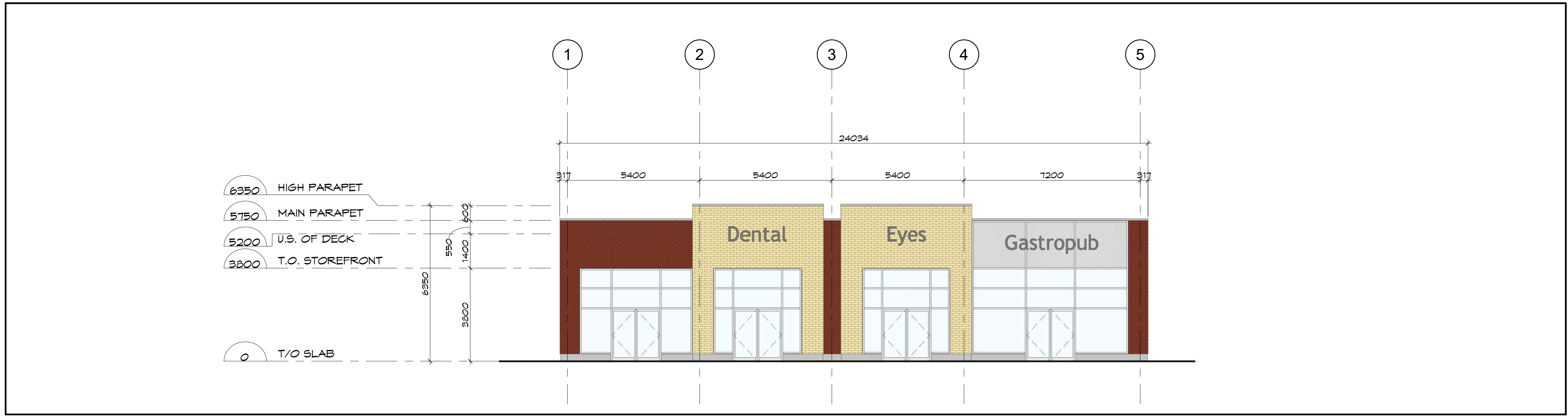
2 ELEVATION @ GRID A (facing parking) A-2 SCALE: 1 : 100
