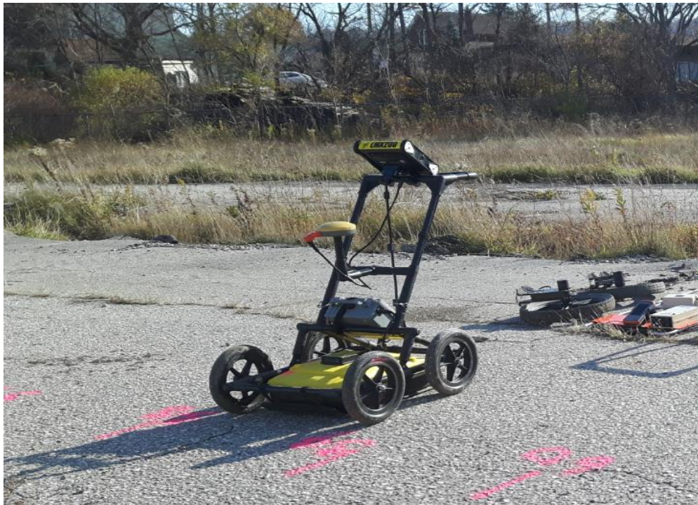
Figure 3: Typical GPR Acquisition System Setup
