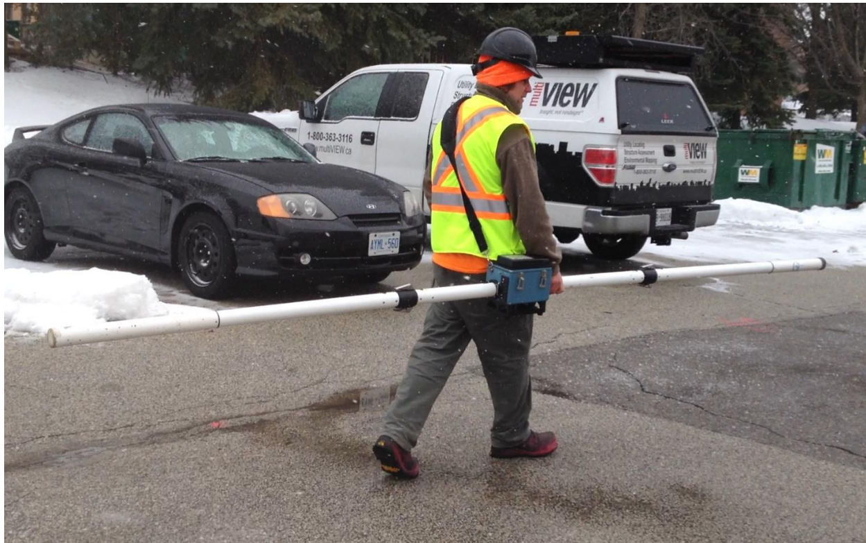
Figure 3-2: Typical FDEM Acquisition System Setup
