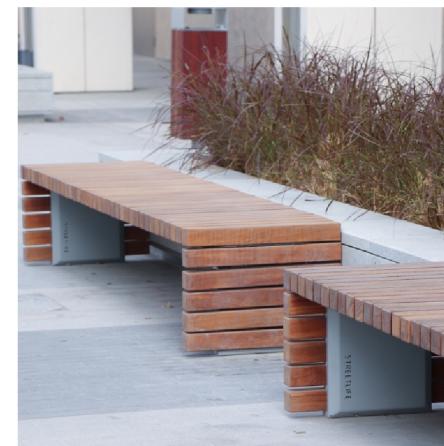
C Solid Staple Benches comprise sturdy, crosswise-positioned Solid slats (7x7 cm – 2.8”x2.8”) on an integrated steel structure. The benches have a slender design, but have a powerful architectural impact. The steel base structure is powder coated in a RAL colour. Despite its slender appearance, the bench is strong and rigid.
