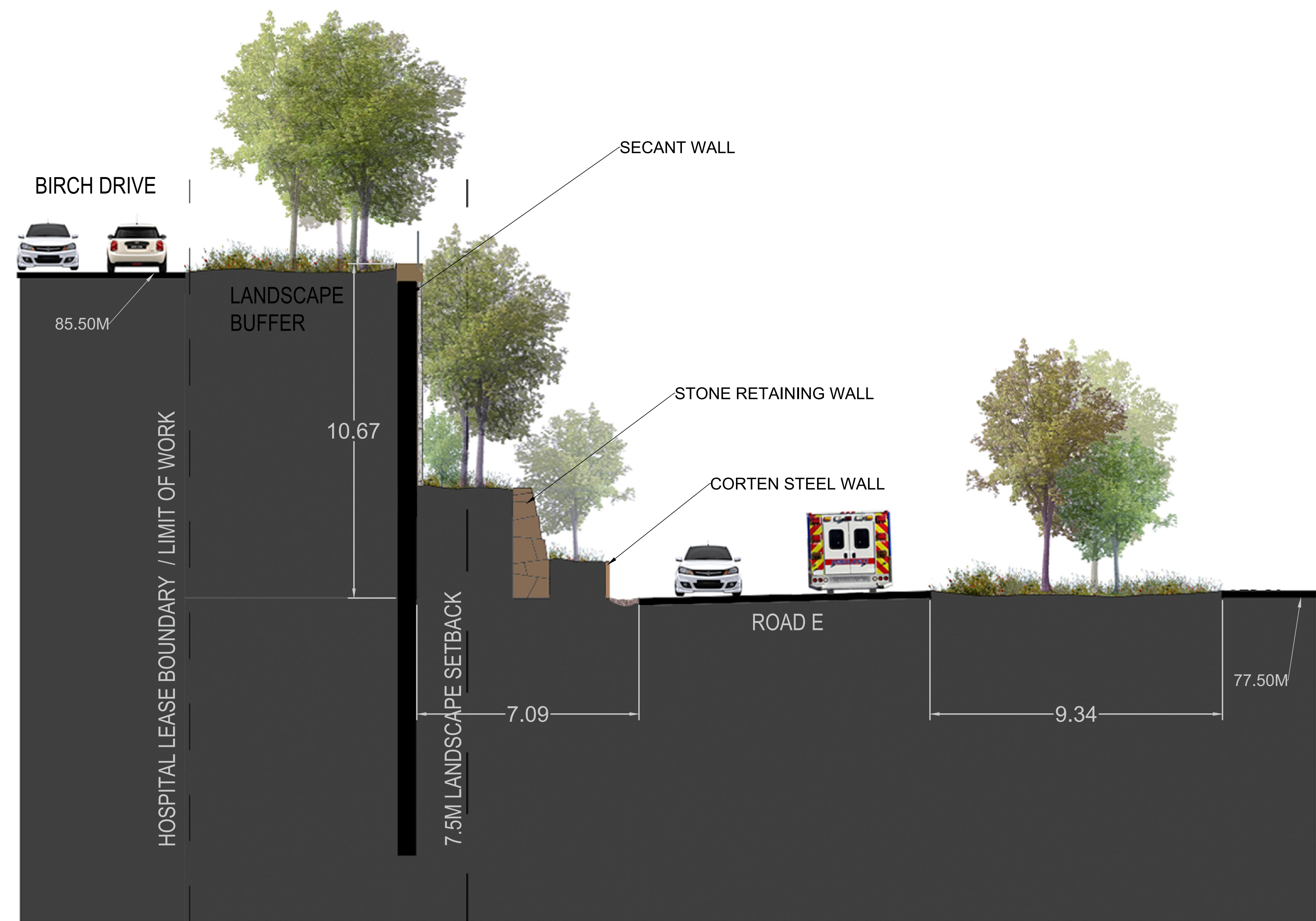
02. ROAD E RETAINING WALL SECTION
