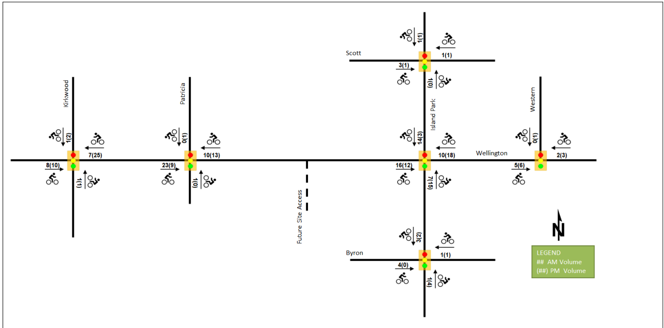
Figure 6: Existing Cyclist Volumes
