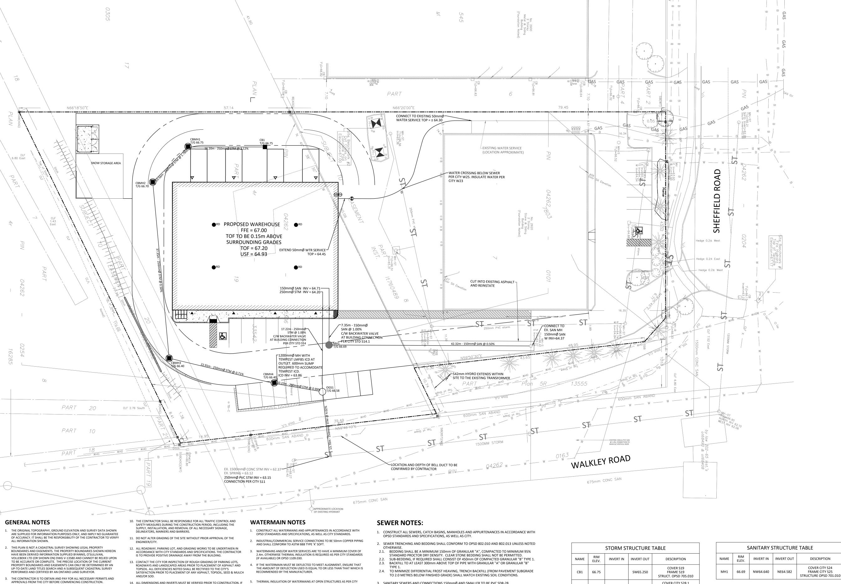
**LOCATION PLAN** — CONCRETE BARRIER CURB — — LIMIT OF CONSTRUCTION CONCRETE WALKWAY PROPOSED ASPHALT STORM SEWER MANHOLE CBMH# CATCHBASIN MANHOLE MH#A SANITARY SEWER MANHOLE → HYD B/F FIRE HYDRANT REMOTE WATER METER ---- 5-YEAR PONDING PROPOSED LANDSCAPING — — 100-YEAR PONDING TACTILE WALKING SURFACE INDICATOR
